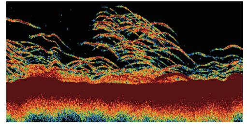
The high level of detail available with TruEcho CHIRP™ technology helps to distinguish fish schools, even when close to the sea bed.
