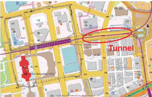
GNSS-only positioning (Positioning interrupted in tunnel)
