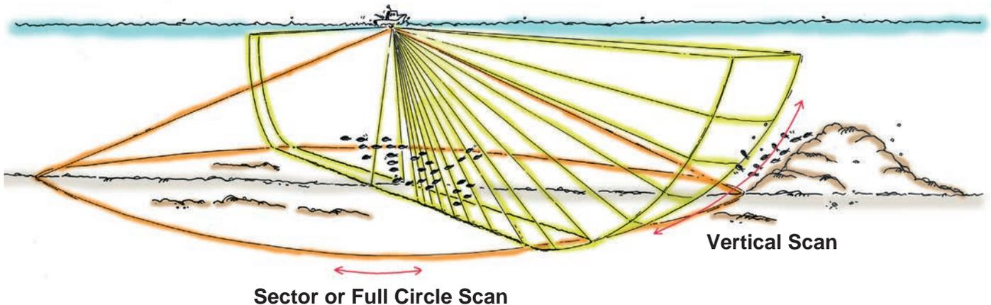
The CH-270 is a sophisticated new searchlight sonar designed for small fishing vessels and pleasure craft. Individual fish, fish schools and underwater objects are displayed on a 10.4" color LCD. The echoes are displayed in 8 or 16 colors according to received echo strength; the strongest echoes are red and the weakest are blue. One echo can be displayed in white so that a specific echo level is highlighted. The background color is also selectable for optimal day and night viewability.
