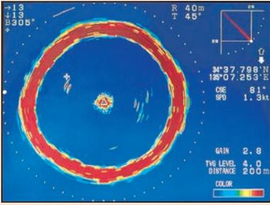
The full circle scan helps to detect fish schools at any bearing around the vessel.
