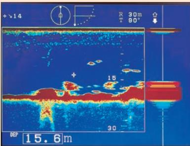
When fully retracted, the transducer tilted to 90 degrees can display fish schools and seabed straight down at high speeds.
