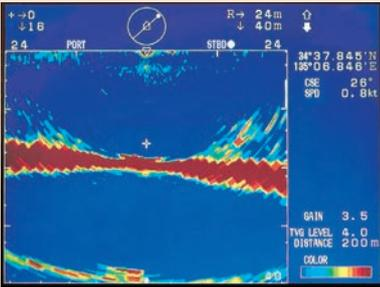
The vertical scan displays the bottom profile within a user-specified vertical plane. The cursor indicator shows range and transducer tilt.
