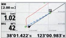
The plotter display traces own ship's track and shows position on a 2-D map\*. This mode presents various data and information with graphic symbols and icons, rather than text. The Auto Waypoint Entry function plots ship's track as "WAYPOINTS". The user may define waypoint entry by time interval, tack angle, etc.
