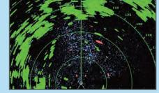
In the unique Rain Mode setting, rain cells are displayed as blue targets and lets you see through a storm cell to identify targets that would normally be hidden in the rain.
