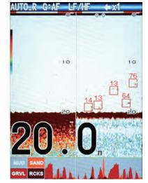
Circles or squares with fish sizes are displayed on fish echoes. When in dual frequencies mode, you can set the mark displayed on both or either frequency screen.
