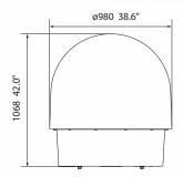
It can also be carried through narrow spaces (800 mm) if disassembled.
