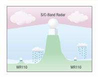
The WR110 can supplement, reinforce and fill-in areas global surveillance weather radars cannot reach.
