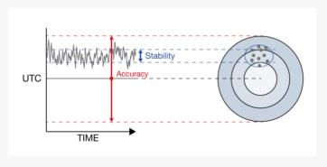
Accuracy refers to the maximum error deviation from UTC true value. Stability refers to the degree of variation from accuracy over a period of time. \* FURUNO defines accuracy on the basis of UTC (vs UTC).
