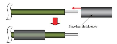
Step 3 Move the heat shrink tubes to the soldered connection, and then apply heat to the tubes.
