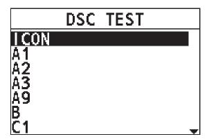
Step 3 Press the **Menu/DSC** control to send the DSC test call. Your radio waits for an acknowledgement from the radio you called.
