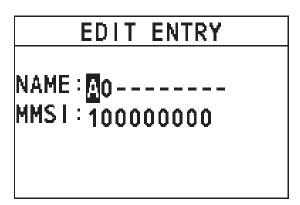
Step 6 After you finish entering the information, press the **Menu/DSC** control to save the setting and return to the previous screen.
