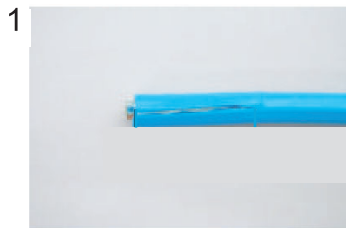
1 Expose inner vinyl sheath.
