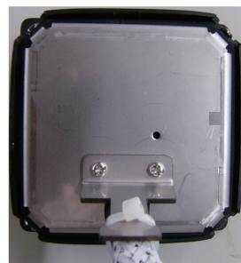
3) Close rear cover. Fasten cable to clamp with cable tie (supplied).
